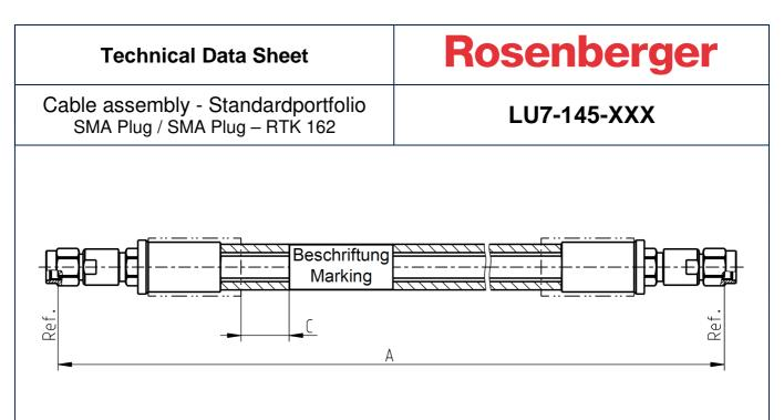
All dimensions are in mm; tolerances according to ISO 2768 c-H
