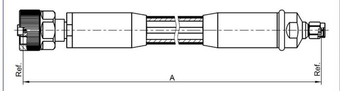
All dimensions are in mm; tolerances:  $\pm$  3mm for A  $\leq$  300 mm;  $\pm$  1% for A > 300 mm
