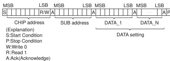
For continuous data transmission, the auto increment function causes data to be written into the sub-address DATA\_(N+1). The sub-address of DATA\_29 is followed by DATA\_1.
