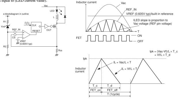
Given that the period when current flows into coil is T c+T d
