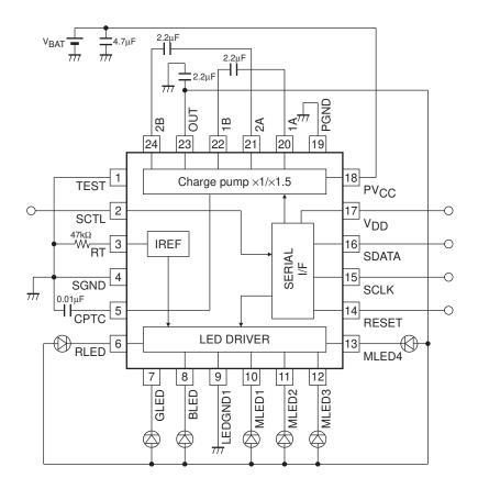
\* The value of the external capacitor connected to the charge pump circuit can be reduced depending on the load current. The minimum rating of the Load current doesn't increase even if  $2.2\mu$ F or more capacitor is used.
