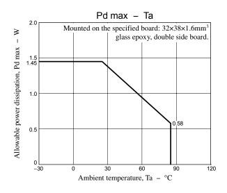
**Specified board** (32mm × 38mm × 1.6mm, glass epoxy, double side board)
