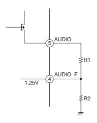
AUDIO\_F is determined by internal band-gap reference voltage (typ = 1.25V).
