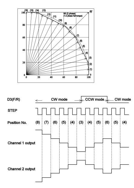
The IC internal D/A converter advances by 1 bits on the rising edge of the input step pulse.
