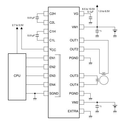
\*1: Connect a kickback absorption capacitor directly near IC. Coil kickback may cause rise of the voltage of VM line, and the voltage exceeding the maximum rating may be applied momentarily, resulting in deterioration or damage of IC.
