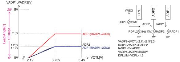
3. The offset and slope can be adjusted as desired by setting RADP1 and RADP12 of ADP1 (pin 15). (It is also possible to set a limit on the lead angle adjustment by means of the CTL voltage by setting DPL.)
