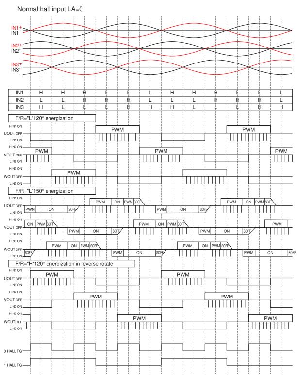
The energization is switched to 120° when 3 Hall FG frequency is 6.1Hz (TYP) or lower A direction of rotation is detected from Hall signal according to F/R pin input If the motor rotates in reverse against F/R pin input, 120° energization is maintained forcibly.
