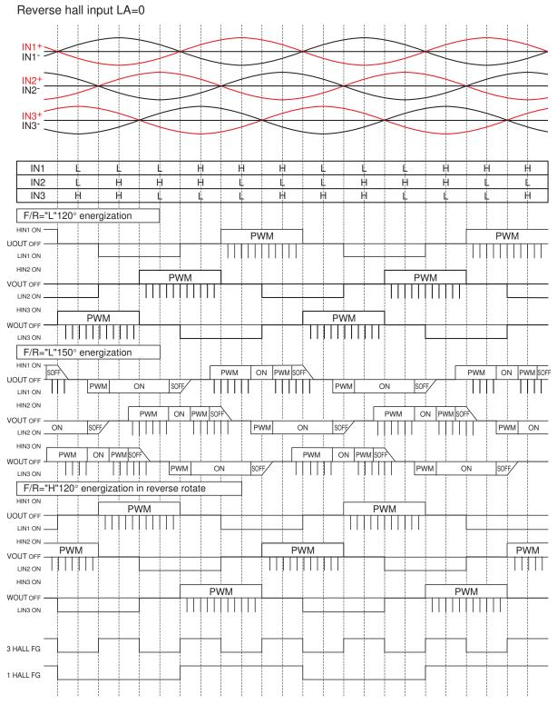
The energization is switched to  $120^{\circ}$  when 3 Hall FG frequency is 6.1Hz (TYP) or lower A direction of rotation is detected from Hall signal according to F/R pin input If the motor rotates in reverse against F/R pin input,  $120^{\circ}$  energization is maintained forcibly.
