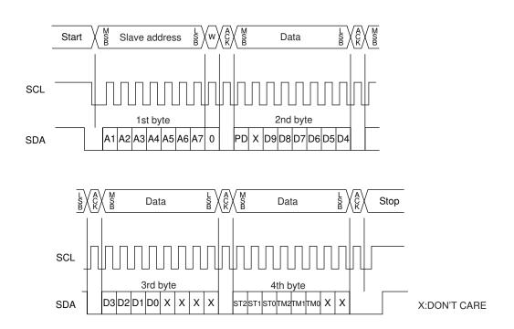
The standard data transfer to this device consists of four bytes: the slave address of the first byte and the data of the second, third and four bytes.
