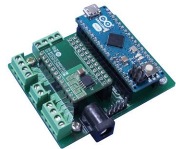
ONBB4AMGEVB Board with Arduino Micro and LV8548MCSLDGEVB Board
