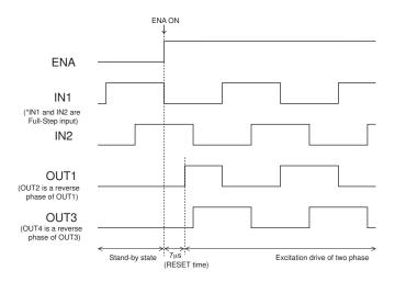
3. Example of current wave type in each excitation mode when stepping motor parallel input is controlled.
