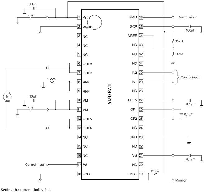
When  $V_{CC} = 5V$ , Vref = 1.5V Ilimit = Vref/5/RNF $= 1.5V/5/0.22\Omega = 1.36A$
