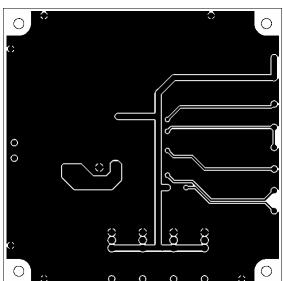
L2 : Copper wiring pattern diagram
