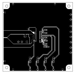
L1 : Copper wiring pattern diagram
