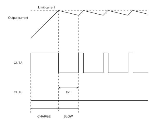
Braking operation time in current limit mode can be set by connecting a capacitor between SCP and GND pins. This setting is the same as the time setting required to turn off the outputs when an output short-circuit occurs as explained in the section entitled "Output Short-circuit Protection Function." See "Output Short-circuit Protection Function," for the setting procedure.
