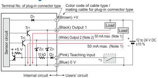
I/O CIRCUIT AND WIRING DIAGRAMS
