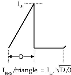
Assuming  $\phi$  is the percentage of allowable input current ripple, C1 can be calculated using the following equations:
