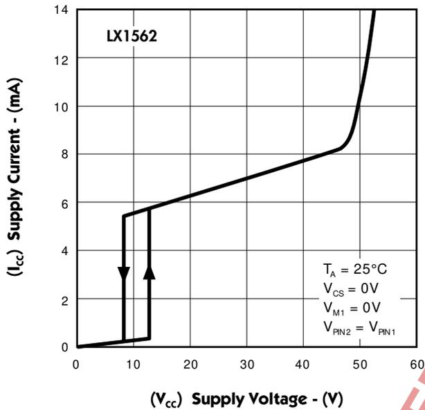
**FIGURE 22.** — SUPPLY CURRENT vs. SUPPLY VOLTAGE
