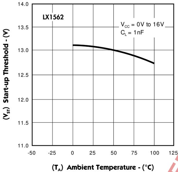
FIGURE 10. — START-UP THRESHOLD vs. TEMPERATURE
