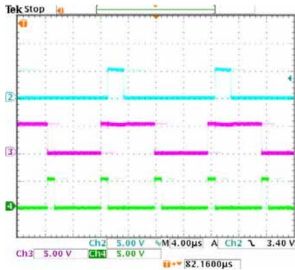
**Figure 3-** Sync signals-Timing relationship to A<sub>OUT</sub>
