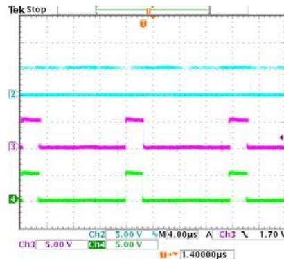
**Figure 5-** Master is in striking mode while slaves are in running mode
