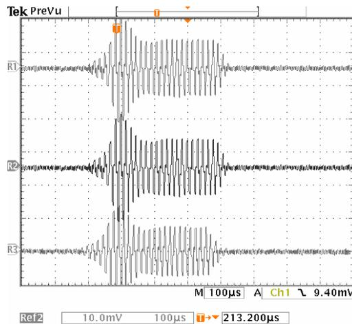
**Figure 8-** Output current during digital dimming with 5% duty cycle R1= i<sub>out</sub>(Master) R2=i<sub>out</sub>(Slave1) R3=i<sub>out</sub>(Slave2) Lamp Current at 10mA/Div
