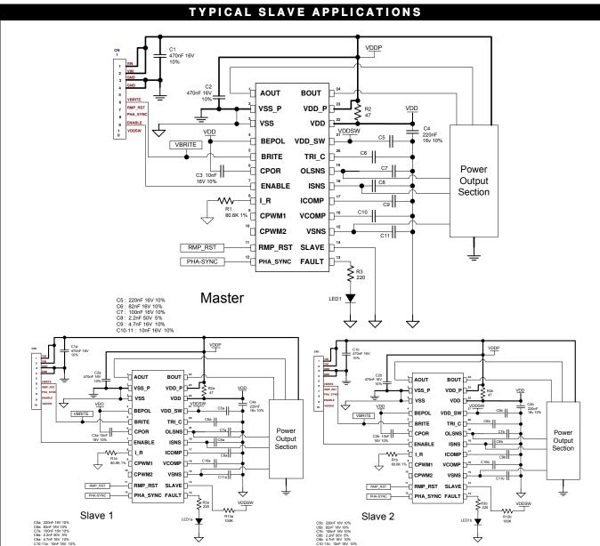
Figure 2 - Schematic Modules Connected as a Master and Slave
