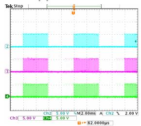
Figure 6- Gate signals during digital dimming with 50% duty cycle CH2= A<sub>OUT</sub>(Master), CH3=A<sub>OUT</sub>(Slave1), CH4=A<sub>OUT</sub>(Slave2)
