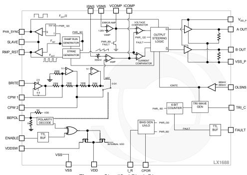
Figure – Simplified Block Diagram
