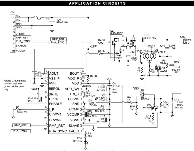
Figure 1 – Schematic for LX1688 Inverter Module Configured as Master
