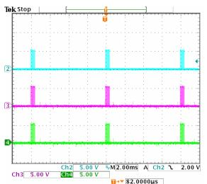
Figure 7- Gate signals during digital dimming with 5% duty cycle CH2= A<sub>OUT</sub>(Master), CH3=A<sub>OUT</sub>(Slave1), CH4=A<sub>OUT</sub>(Slave2)
