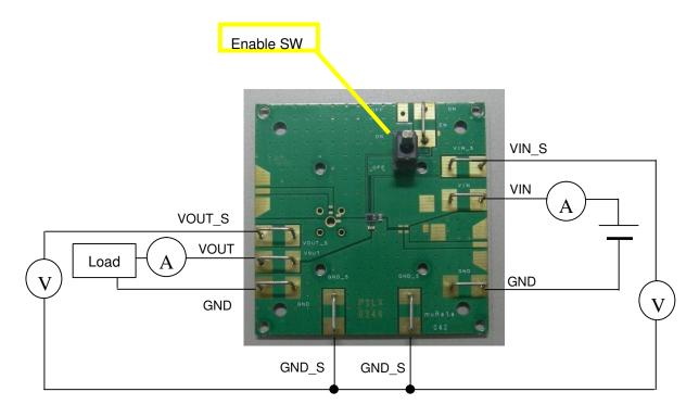
The enable switch has three positions.
