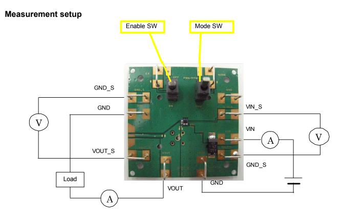
The enable switch has three positions.
