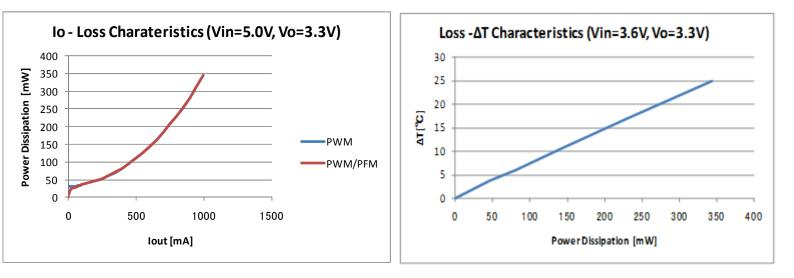
The output current of the device may need to be de-rated if it is operated in high ambient temperature or in an application that requires continuous power delivery. The amount of current de-rating is highly dependent on the environmental thermal conditions, e.g., PCB design, nearby components, or effective air flow. Care should especially be taken in applications where the device temperature exceeds 85°C.
