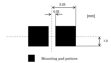
4-3. Recommended mounting pattern at antenna side for the attachment by adhesive
