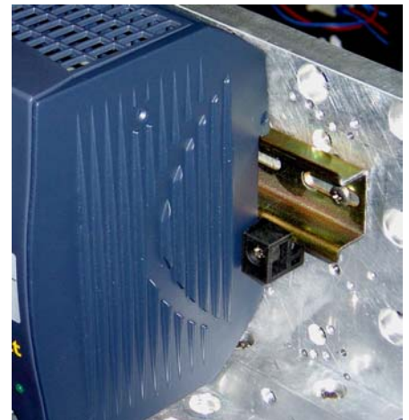
Fig. 23 One of four DIN-rail fixing brackets HZZ00624-G (DMB-EWG)
