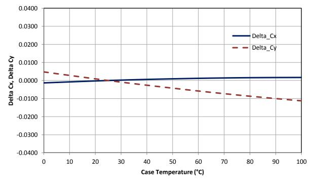
Figure 9: Typical chromaticity coordinate shift vs. Case temperature  $% \left( 1\right) =\left( 1\right) \left( 1\right$
