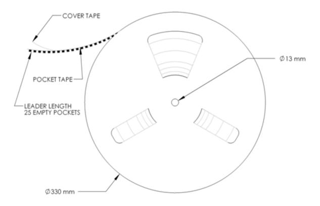
Figure 13: Emitter Reel specifications (mm).
