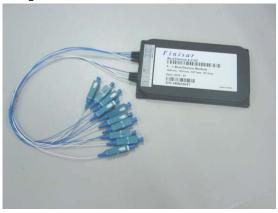
The Finisar MUX/DEMUX-4-2 optibox module is a passive optical multiplexer/ demultiplexer designed for metro access applications that represents the state of the art in fiber optics design. The MUX/DEMUX-4-2 optibox module multiplexes and demultiplexes four CWDM wavelength channels from a two-fiber circuit. Finisar's design allows the creation of cost-effective unidirectional network traffic rings or point-to-point
