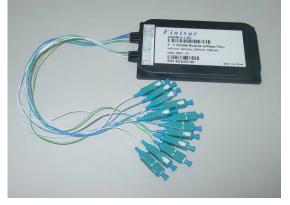
The Finisar MUX/DEMUX-4-EX optibox module is a passive optical multiplexer/demultiplexer designed for metro access applications that represents the state of the art in fiber optics design. The MUX/DEMUX-4-EX optibox module multiplexes and demultiplexes four CWDM wavelength channels from a two-fiber circuit and passes the other channels. Finisar's design allows the creation of cost-effective unidirectional network traffic rings or point-to-point links.
