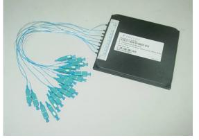
The Finisar MUX/DEMUX-8 optibox module is a passive optical multiplexer/ demultiplexer designed for metro access applications that represents the state of the art in fiber optics design. The MUX/DEMUX-8 optibox module multiplexes and demultiplexes eight CWDM wavelength channels from a two-fiber circuit. Finisar's design allows the creation of cost-effective unidirectional network traffic rings or point-to-point links.
