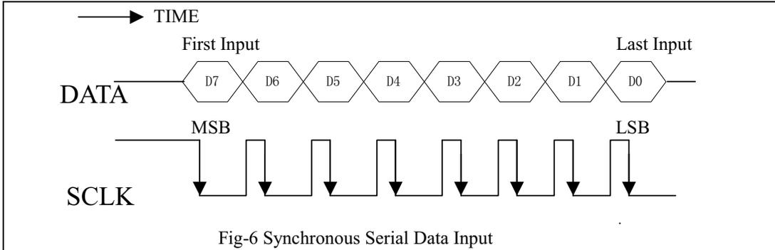
Fig-6 Synchronous Serial Data Input
