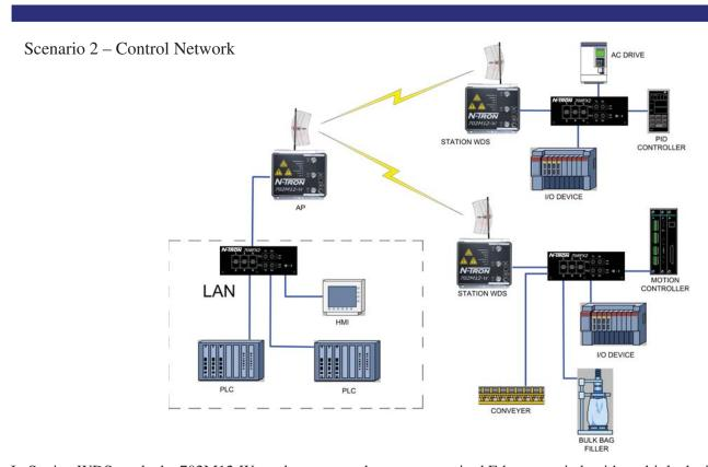
In Station WDS mode the 702M12-W can be connected to a remote wired Ethernet switch with multiple devices connected to the switch.
