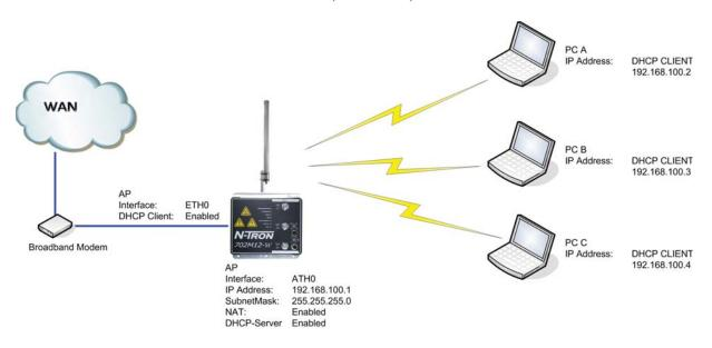
The N-TRON 702M12-W configured as a router can act as a DHCP server and supports the Network Address Translation (Masquerading) feature which is widely used by Access Points. This automates the assigning of IP addresses to devices as they connect. NAT will act as a firewall between LAN and WLAN networks. Additional firewall settings can be configured for layer 3 packet filtering and access control in Router mode.
