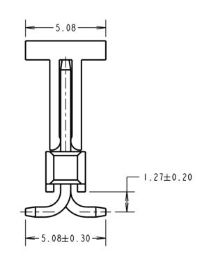
SPECIFICATION: MATERIAL: MOULDING = NYLON 6T UL94V-0, BLACK CONTACT = BRASS FINISH:
