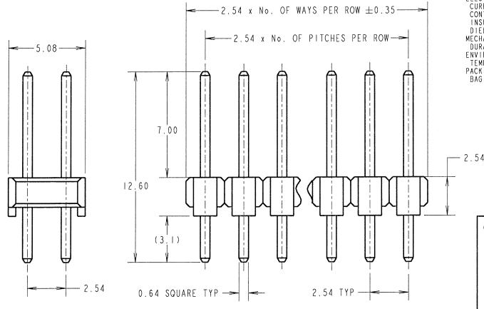
MOULDING = HIGH TEMP NYLON 6T UL94V-O, BLACK PINS = BRASS FINISH: PINS: 45 = GOLD 46 = 100% TIN OVER NICKEL ELECTRICAL: CURRENT RATING = 3A MAX CONTACT RESISTANCE = 25 m $\Omega$  MAX (GOLD), 30 m $\Omega$  MAX (TIN) INSULATION RESISTANCE = 1.000 M $\Omega$  MIN DIELECTRIC STRENGTH = 750V AC/DC MECHANICAL: DURABILITY = 300 OPERATIONS (GOLD), 50 OPERATIONS (TIN) ENVIRONMENTAL: TEMPERATURE RANGE = -40°C TO +105°C PACKING: BAG
