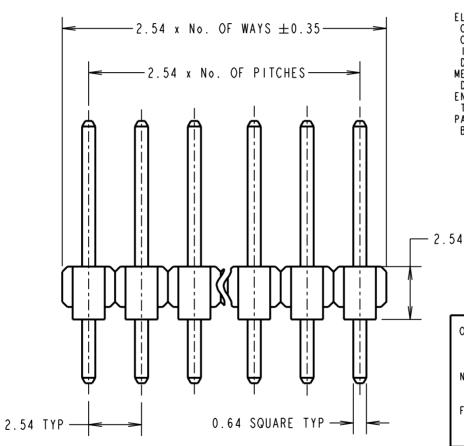
MATERIAL: MOULDING = HIGH TEMP NYLON 6T UL94V-O. BLACK PINS = BRASS FINISH: PINS: 45 = GOLD 46 = 100% TIN OVER NICKEL ELECTRICAL: CURRENT RATING = 3A MAX CONTACT RESISTANCE = 25 m $\Omega$  MAX (GOLD), 30 m $\Omega$  MAX (TIN) INSULATION RESISTANCE = 1,000  $M\Omega$  MIN DIELECTRIC STRENGTH = 750V AC/DC MECHANICAL: DURABILITY = 300 OPERATIONS (GOLD), 50 OPERATIONS (TIN) ENVIRONMENTAL: TEMPERATURE RANGE = -40°C TO +105°C PACKING: BAG
