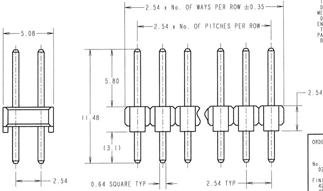
MATERIAL: MOULDING = HIGH TEMP NYLON 6T UL94V-O, BLACK PINS = BRASS FINISH: PINS: 42 = GOLD ON CONTACT AREA, 100% TIN ON TAILS 46 = 100% TIN OVER NICKEL ELECTRICAL: CURRENT RATING = 3A MAX CONTACT RESISTANCE = 25 m $\Omega$  MAX (GOLD), 30 m $\Omega$  MAX (TIN) INSULATION RESISTANCE = 1.000 M $\Omega$  MIN DIELECTRIC STRENGTH = 750V AC/DC DURABILITY = 300 OPERATIONS (GOLD), 50 OPERATIONS (TIN) FNVIRONMENTAL: TEMPERATURE RANGE = -40°C TO +105°C PACKING: BAG
