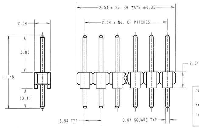
MATERIAL: MOULDING = HIGH TEMP NYLON 6T UL94V-0, BLACK PINS = BRASS FINISH: PINS: 42 = GOLD ON CONTACT AREA, 100% TIN ON TAILS 46 = 100% TIN OVER NICKEL ELECTRICAL: CURRENT RATING = 3A MAX CONTACT RESISTANCE = 25 m $\Omega$  MAX (GOLD), 30 m $\Omega$  MAX (TIN) INSULATION RESISTANCE = 1,000 M $\Omega$  MIN DIELECTRIC STRENGTH = 750V AC/DC MECHANICAL: DURABILITY = 300 OPERATIONS (GOLD), 50 OPERATIONS (TIN) FNVIRONMENTAL: TEMPERATURE RANGE = -40°C TO +105°C PACKING: BAG
