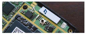
These highly innovative antennas provide competitive advantages for designers of cell phones, laptops and other mobile equipment by combining GPS & Bluetooth antennas in a single, highly compact form factor suitable for the thinnest/smallest devices. Ethertronics Isolated Magnetic Dipole (IMD) technology utilizes superior RF isolation to deliver the utmost in high performance.
