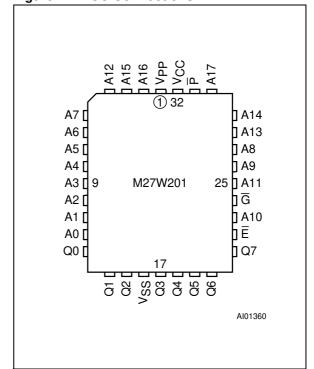
Figure 2C. TSOP Connections
