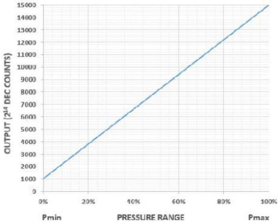
$$\text{OUTPUT (DECIMAL COUNTS)} = \frac{15000-1000}{P_{\text{max}} - P_{\text{min}}} \times (P_{\text{applied}} - P_{\text{min}}) + 1000$$
