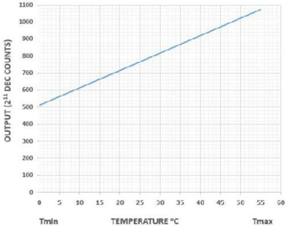
$$\text{OUTPUT (DECIMAL COUNTS)} = \frac{(\text{OUTPUT}^{\circ\text{C}} + 50^{\circ\text{C}}) \times 2048}{150^{\circ\text{C}} - (-50^{\circ\text{C}})}$$
