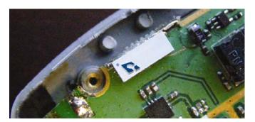
Ethertronics' Savvi series of Isolated Magnetic Dipole<sup>TM</sup>(IMD) antennas deliver on the key needs of device designers for higher functionality and performance in smaller/thinner designs. These innovative antennas provide compelling advantages for GPS enabled cell phones, navigation equipment, and other mobile devices.
