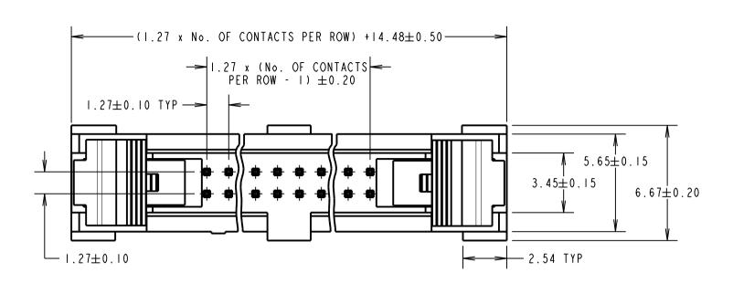
SPECIFICATIONS: MATERIALS: MOULD = LCP, 30% G/F, UL94V-0 CONTACT = BRASS 42 = 0.015-0.02μ GOLD ON CONTACTS, 2.54μ 100% TIN ON TAILS, OVER 0.76-2.03μ NICKEL MECHANICAL: DURABILITY = 300 CYCLES MIN
