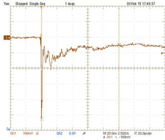
Figure 2. IEC61000-4-2 -8kV Contact ESD Clamping Voltage
