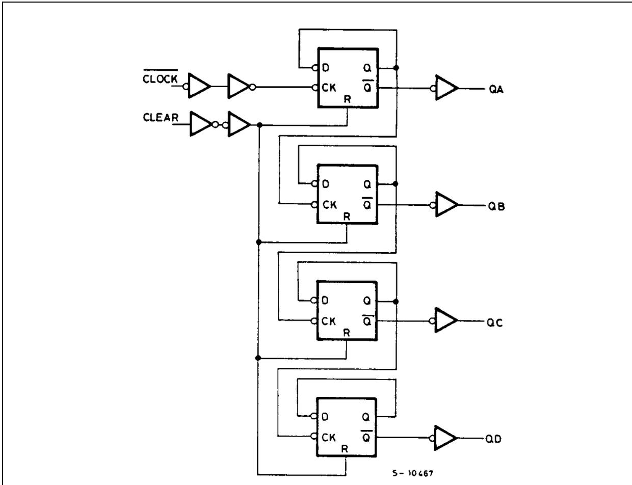
This logic diagram has not be used to estimate propagation delays
