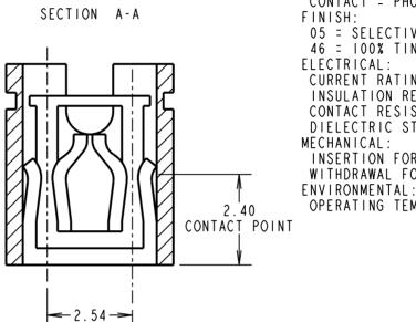
MATERIAL: INSULATOR = 30% GLASS FILLED PBT UL94V-0 (SEE ORDER CODE FOR COLOUR) CONTACT = PHOSPHOR BRON7F FINISH: 05 = SELECTIVE GOLD OVER NICKEL 46 = 100% TIN ELECTRICAL: CURRENT RATING = IA INSULATION RESISTANCE = 5,000 MEGOHMS MIN CONTACT RESISTANCE = 20 MILLIOHMS MAX DIELECTRIC STRENGTH = 500V AC MECHANICAL:
