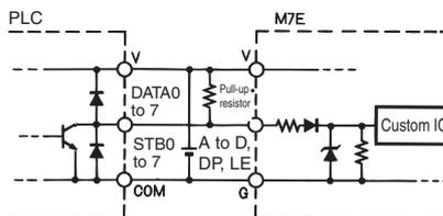
Note: 1. Supply 24 VDC only. The PLC does not operate with the M7E Negative Logic Model.
