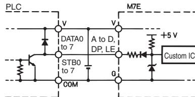
2. Connected to C200H-OD215 Transistor Output Unit \*2 \*3
