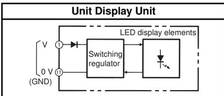
**Note:** The terminal numbers of the Unit Display Unit are different from the terminal numbers of the connector. Refer to *Terminal Arrangements and Functions* on page 3 for details.
