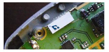
Ethertronics' Savvi series of Isolated Magnetic Dipole  $^{TM}(IMD)$  antennas deliver on the key needs of device designers for higher functionality and performance in smaller/thinner designs. These innovative antennas provide compelling advantages for GPS enabled cell phones, navigation equipment, and other mobile devices.
