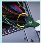
Flexible clamp jaw easily wraps around bus bars and cable bundles that may be difficult to access with regular clamp meters. The thin 7.5mm cable diameter easily fits into tight spaces. Choose between a 10" (25.4cm) or 18" (45.7cm) cable clamp length to accommodate your application needs.
