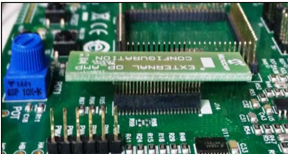
FIGURE 1: EXTERNAL OP AMP CONFIGURATION BOARD
