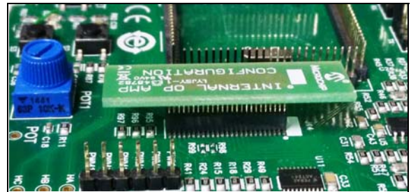
FIGURE 2: INTERNAL OP AMP CONFIGURATION BOARD
