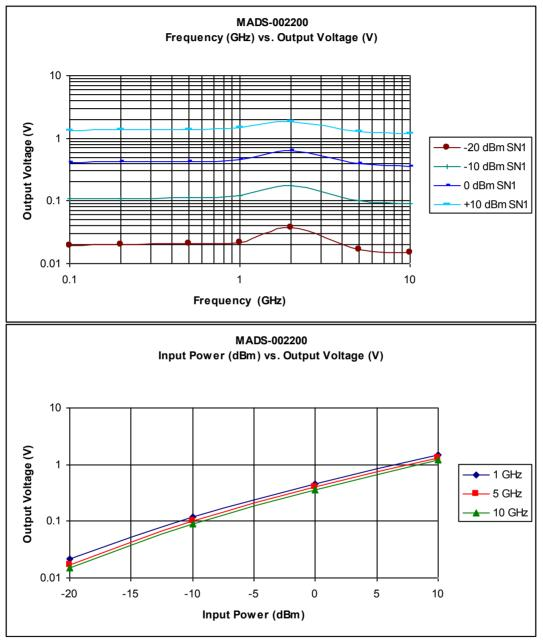
The MADS-002200 in an SC-79 Package Style was evaluated in a detector circuit in which the Schottky diode terminates a 50 Ohm transmission line on a duroid substrate. The SC-79 packaged diode was attached to the terminal of a 3.5mm connector and the output voltage was measured through a bias tee on a voltmeter. Matching was not attempted.
