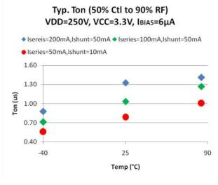
Typ. Ton (50% Ctl to 90% RF) vs. VDD VCC=3.3V, IBIAS=6μA Iseries=200mA, Ishunt=50mA
