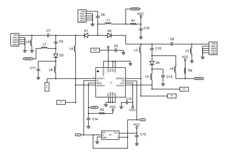
14. This is the schematic of MADR-010547-001SMB. The frequency range for this application circuit is 200 MHz to 500 MHz. The bias current for the series diodes is 200 mA. The bias current for the shunt diodes is 50 mA. The recommended inductors are Coil Craft 0603LS-181XJLB for both current and frequency considerations. For different frequency applications, both capacitors and inductors should be adjusted accordingly.
