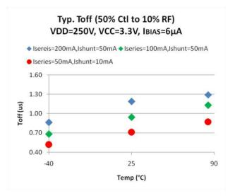
Typ. Toff (50% Ctl to 10% RF) vs. VDD VCC=3.3V, IBIAS=6μA Iseries=200mA, Ishunt=50mA
