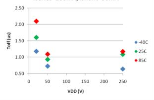
The switch is a series/shunt, series/shunt SPDT switch using four M/A-COM MA4P504-1072T PIN diodes. Schematic is on next page. Switching parameters were measured with 500 MHz 20W CW RF signal.
