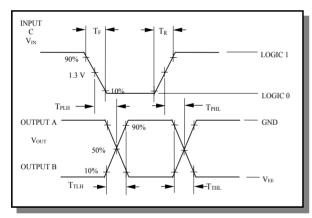
Note: See Switching Wave Forms for the definition of the switching terms. Supplies must be by-passed with .01 µF Capacitors.
