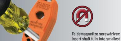
Insert shaft fully into smallest demagnetizing slot that fits; avoid rotating shaft while drawing out slowly
