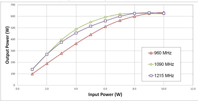
**RF** Power Transfer Curve (Output Power Vs. Input Power)
