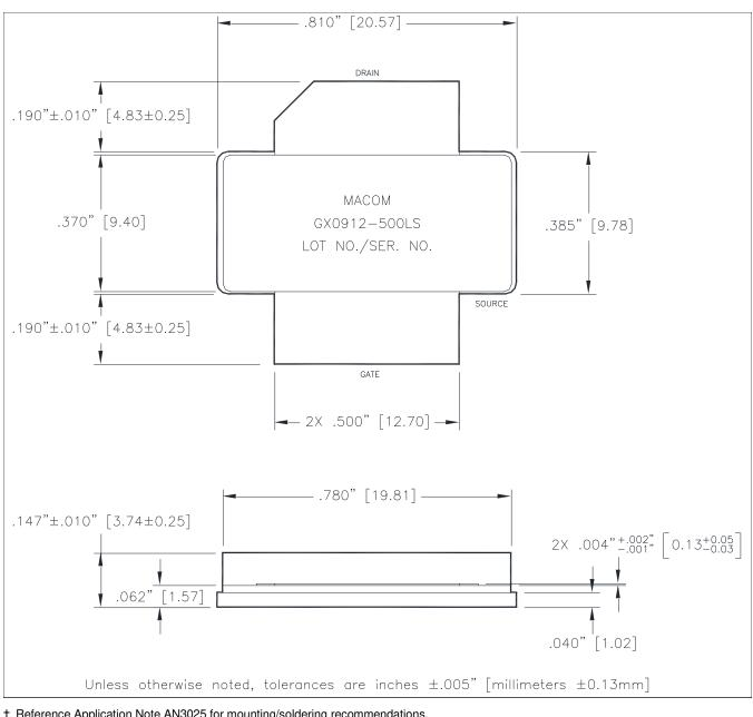
† Reference Application Note AN3025 for mounting/soldering recommendations. Meets JEDEC moisture sensitivity level 1 requirements. Plating is Ni/Au. МЛСОМ
